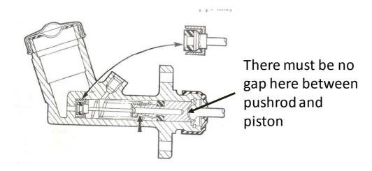
Having identified this, I restored the end of the pushrod to the extent that the instant the clutch pedal is pressed, the pushrod makes contact with the piston, thus eliminating any wastage of valuable pedal stroke. I am pleased to report that the clutch engagement point is now about 1/3 of the way up from the floor which is probably about right and won't over-throw the clutch spring unit.
